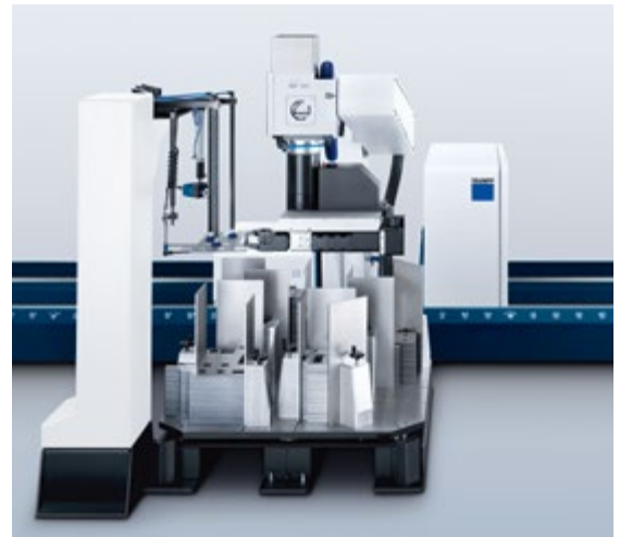
Sheet removal station with rotary table
