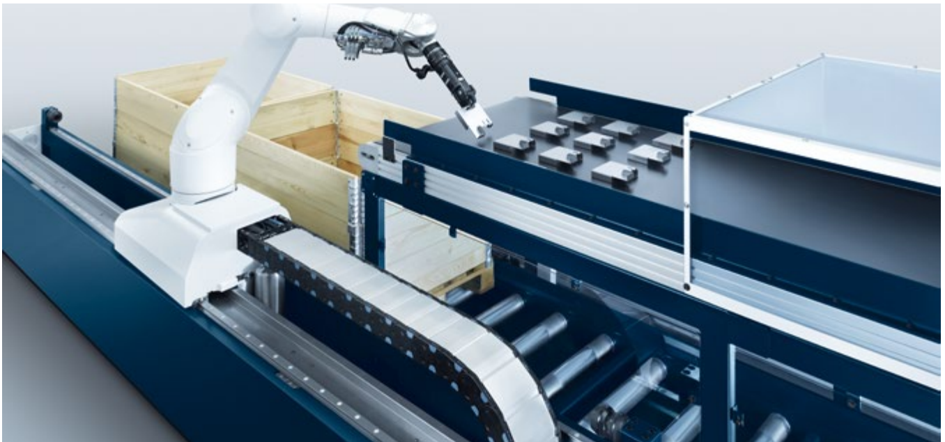
Conveyor system with conveyor belt and pallet conveyor
