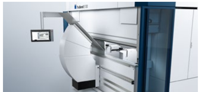
The bending aid – supports the operator.
