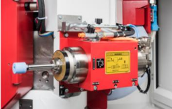
The swiveling wheelhead is equipped with water-cooled, roller-based, and maintenance-free motor spindles with stepless speed control and the latest generation of contact sensors. The shaft ends hold external wheelheads with a diameter of 500 mm (20") and a width of 63 (80 F5) mm (2.48" (3.15" F5)). For internal grinding, use powerful high-frequency spindles with 120 mm (4.72") external diameter. It's your choice: configure the wheelhead to match your specific needs.
