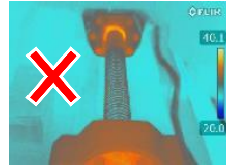
without ball screw cooling
