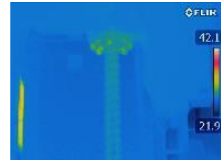
with ball screw cooling (Makino)
