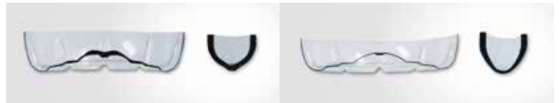
Influence of different preform domes on bottle bases
