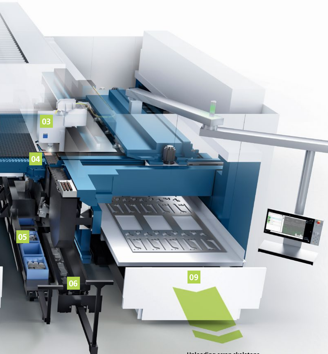
Unloading scrap skeletons
